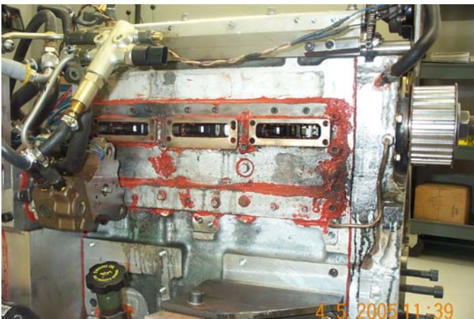
Figure 5 – Teardown of the test engine to improve leaking intake runners and exhaust manifold.
