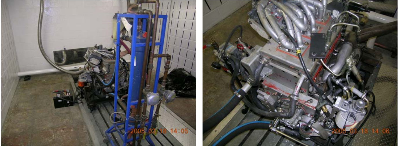
Figure 3 – LIM 353 engine set up in test cell. Dynamometer not used for initial idle testing.
