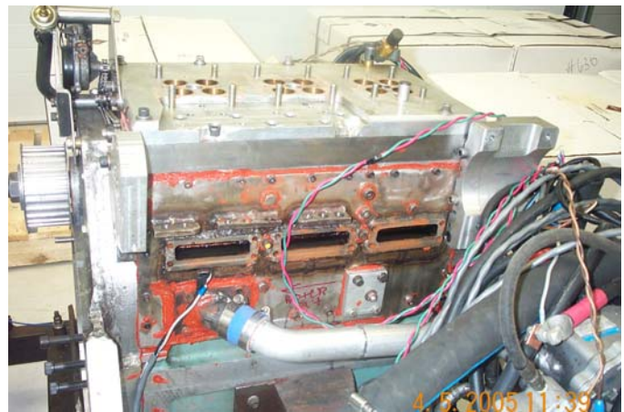
Figure 5 – Teardown of the test engine to improve leaking intake runners and exhaust manifold.
